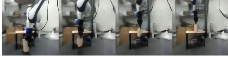
(a) Comparing accuracy of predictions to ground truth trajectory. (Top Row) Video frames of a ground-truth trajectory from a robot in our lab. (Middle row) Each frame is encoded by V-JEPA 2 encoder, and then decoded using the feedforward frame decoder. Reconstructions of the V-JEPA 2 representations show that the encoder captures the salient parts of the scene necessary for vision-based control; blurry background generation can be partially attributed to the low-capacity of our feedforward frame decoder. (Bottom Row) Autoregressive rollout produced by V-JEPA 2-AC world model using the ground-truth action sequence given first frame as context, and then decoded using feedforward frame decoder. Reconstructions of the V-JEPA 2-AC rollout show that the action-conditioned world model successfully animates the robot while keeping the background and non-interacted objects (e.g., the shelf) unaffected. However, we do observe error accumulation as the world model predicts the location of the cup to be slightly lower than that of the real trajectory in the final frame.
